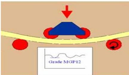
The stress placed on the timber is usually on its Minor Axis.
