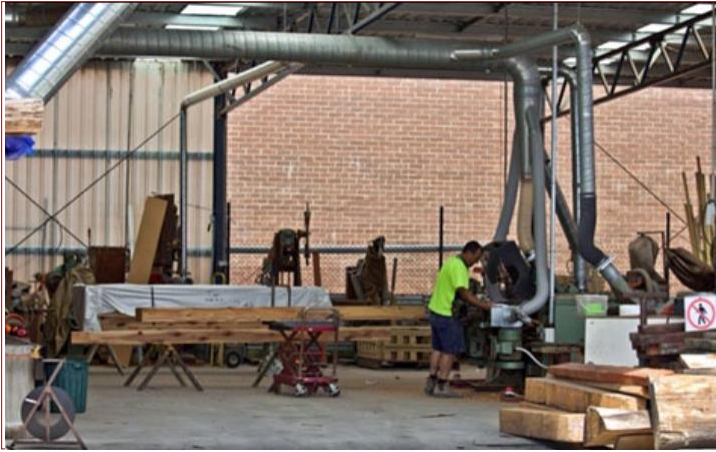
Cypress being dressed with a 4-sided thicknesser
