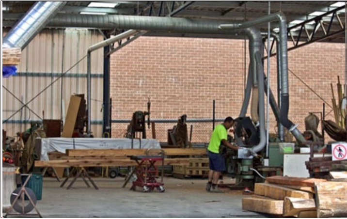
Cypress being dressed with a 4-sided thicknesser
