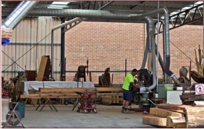
Cypress being dressed with a 4-sided thicknesser
